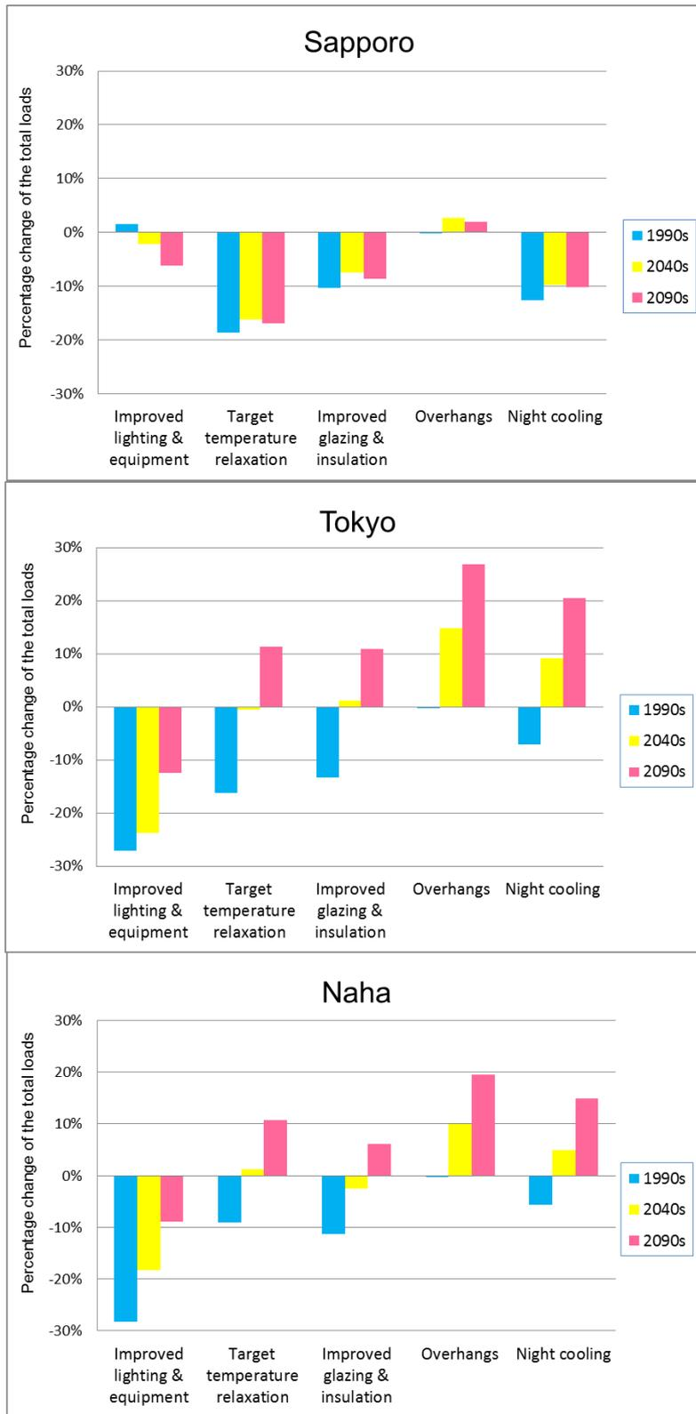
Fig 5.17 Percentage change of the total heating/cooling loads by each strategy compared to the 1990s base model
