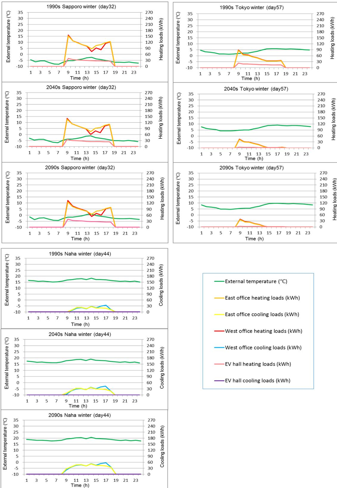
Fig 5.21 Heating/cooling loads profile of the cumulatively improved model on a typical winter day
