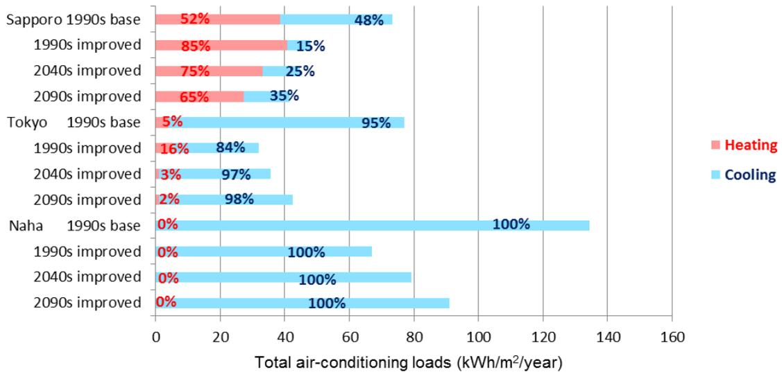
Fig 5.19 Heating/cooling load comparison between the cumulatively improved model and the 1990s base model
