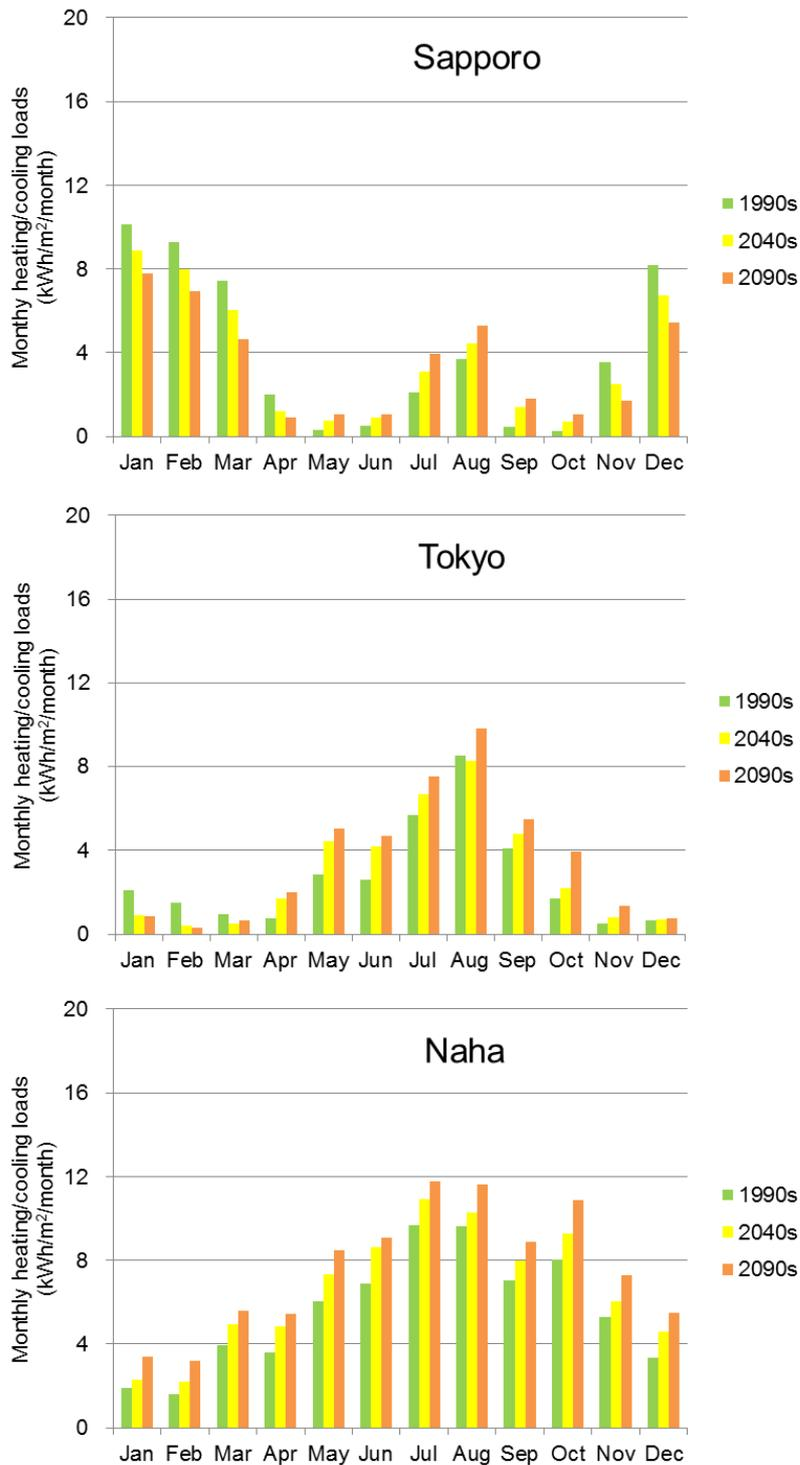
Fig 5.23 Monthly heating/cooling load of the cumulatively improved model
