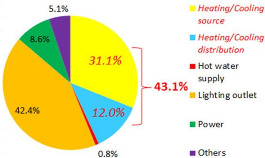
Fig 2.9 Energy consumption percentage of a tenant building with a rentable ratio of more than 60% in Japan (ECCJ 2011a)
