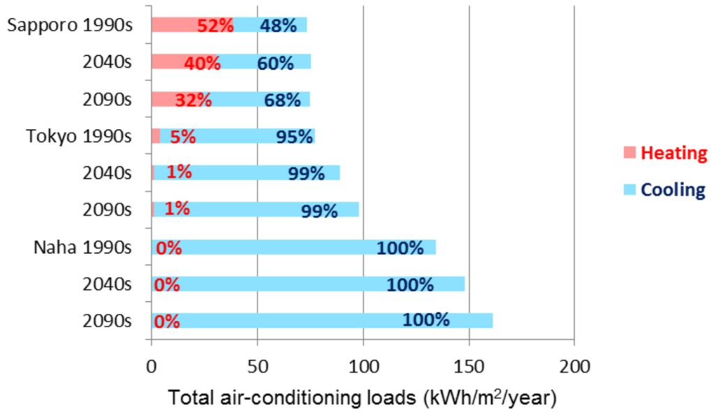
Fig 5.2 Heating/cooling loads of the base model
