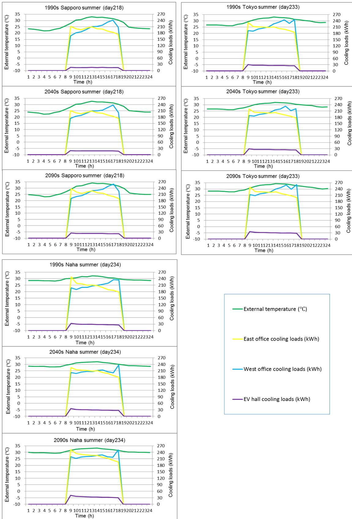
Fig 5.5 Cooling loads profile of the base model on a typical summer day
