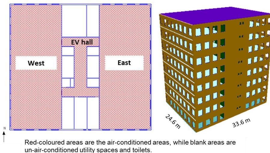
Fig 4.6 Office building model and zoning for typical 1990s type buildings (a representative floor plan and outward)
